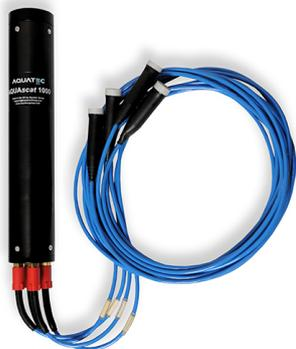
The AQUAscat® 1000R is an acoustic suspended sediment profiler specially designed and manufactured as a research model. 4 cabled transducers are supplied with the instrument, each of which transmits short pulses of ultrasound, which are then scattered back by the sediment in the
